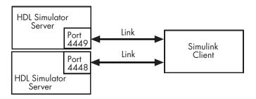
When you link the HDL simulator with a Simulink application, the simulator functions as the server. Using the EDA Simulator Link IN communications interface, an HDL Cosimulation block cosimulates a hardware component by applying input signals to and reading output signals from an HDL model under simulation in the HDL simulator.
