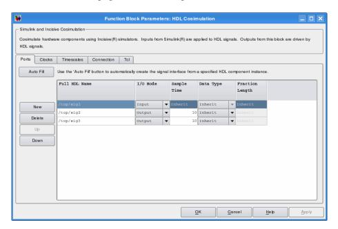
• Connection Pane: Type of communication and communication settings to be used for exchanging data between simulators. See "Connection Pane" on page 6-10 in the Chapter 6, "Simulink Block Reference".
