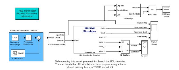
The HDL Cosimulation block models a Manchester receiver that is coded in HDL. Other blocks and subsystems in the model include the following:
