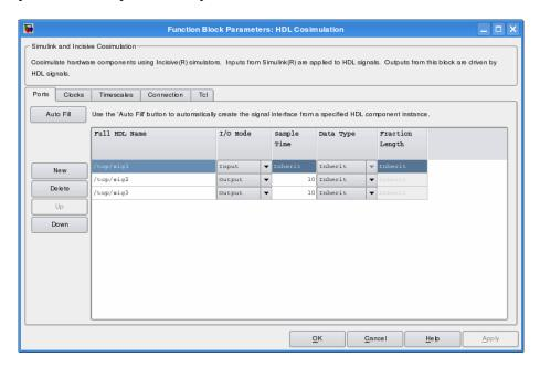
The list at the center of the pane displays HDL signals corresponding to ports on the HDL Cosimulation block.
