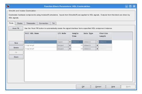
In this pane, you define the HDL signals of your design that you want to include in your Simulink block and set a sample time and data type for output ports. The parameters that you should specify on the **Ports** pane depend on the type of device the block is modeling as follows:
