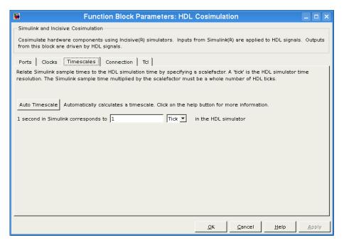
The **Timescales** pane specifies a correspondence between one second of Simulink time and some quantity of HDL simulator time. This quantity of HDL simulator time can be expressed in one of the following ways:
