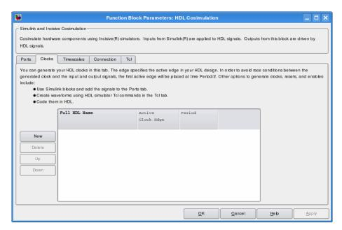
The scrolling list at the center of the pane displays HDL clocks that drive values to the HDL signals that you are modeling, using the deposit method.
