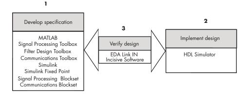
As the figure shows, EDA Simulator Link IN software connects tools that traditionally have been used discretely to perform specific steps in the design process. By connecting these tools, the link simplifies verification by allowing you to cosimulate the implementation and original specification directly. This cosimulation results in significant time savings and the elimination of errors inherent to manual comparison and inspection.
